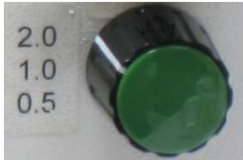
The Weight Selection Dial showing 0.5, 1 and 2 psi.
